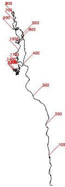
Figure 5: A path of the underwater vehicle was plotted using the images and sonar data. The image frame numbers along the path is shown with selected images (Original data derived from [Williams and Mahon, 2004] and processed into graph form by the present authors).
